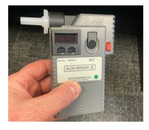
Running a Test - The Alco-Sensor IV product line has a one-way mouthpiece that is inserted into the instrument to turn the instrument on. The mouthpiece allows the subject to provide a sample for analysis. The mouthpiece is a large portion of the breath sample path, and the check valve in the mouthpiece reduces the likelihood that a subject will draw an inhaled breath sample, from the instrument, back through the mouthpiece. Use of a barrier filtered mouthpiece adapter can further reduce the
