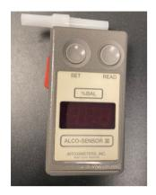
The Alco-Sensor and Alco-Sensor III product lines have a single nipple that the mouthpiece attaches to. The mouthpiece is effectively the entire sample path for the provided breath sample.
