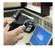
The Alco-Sensor FST and Alco-Sensor V<sub>XL</sub> products have two nipples that a mouthpiece attaches to. The mouthpieces are effectively the entire sample path. The mouthpiece for these instruments are designed to direct the breath out the top of the mouthpiece. Use of a barrier filtered mouthpiece adapter can further reduce the likelihood of disease transmission or instrument contamination.
