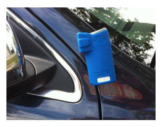
Magnets on both sides of the instrument strongly adhere to ferrous metal surfaces such as a car, to prevent instrument loss during the heat of an arrest.
